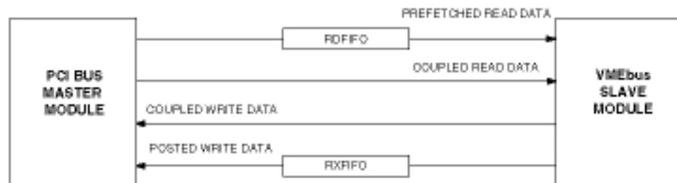
Figure 8-1 VMEbus Slave Channel Dataflow
