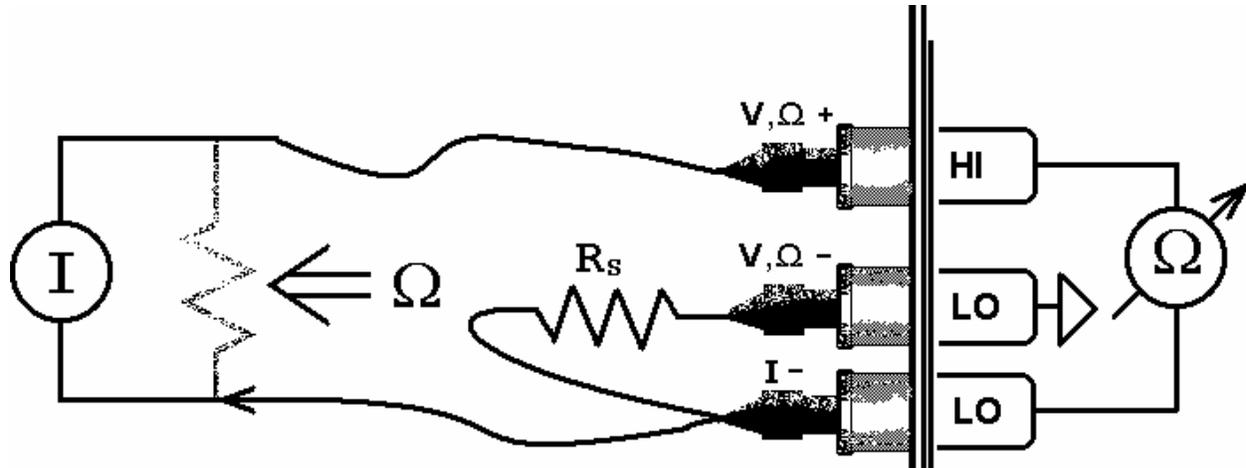
Figure 4-18. Synthesizing resistance into a current source.
