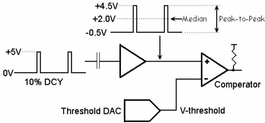
Figure 4-11. AC coupled timing measurements with Threshold DAC.
