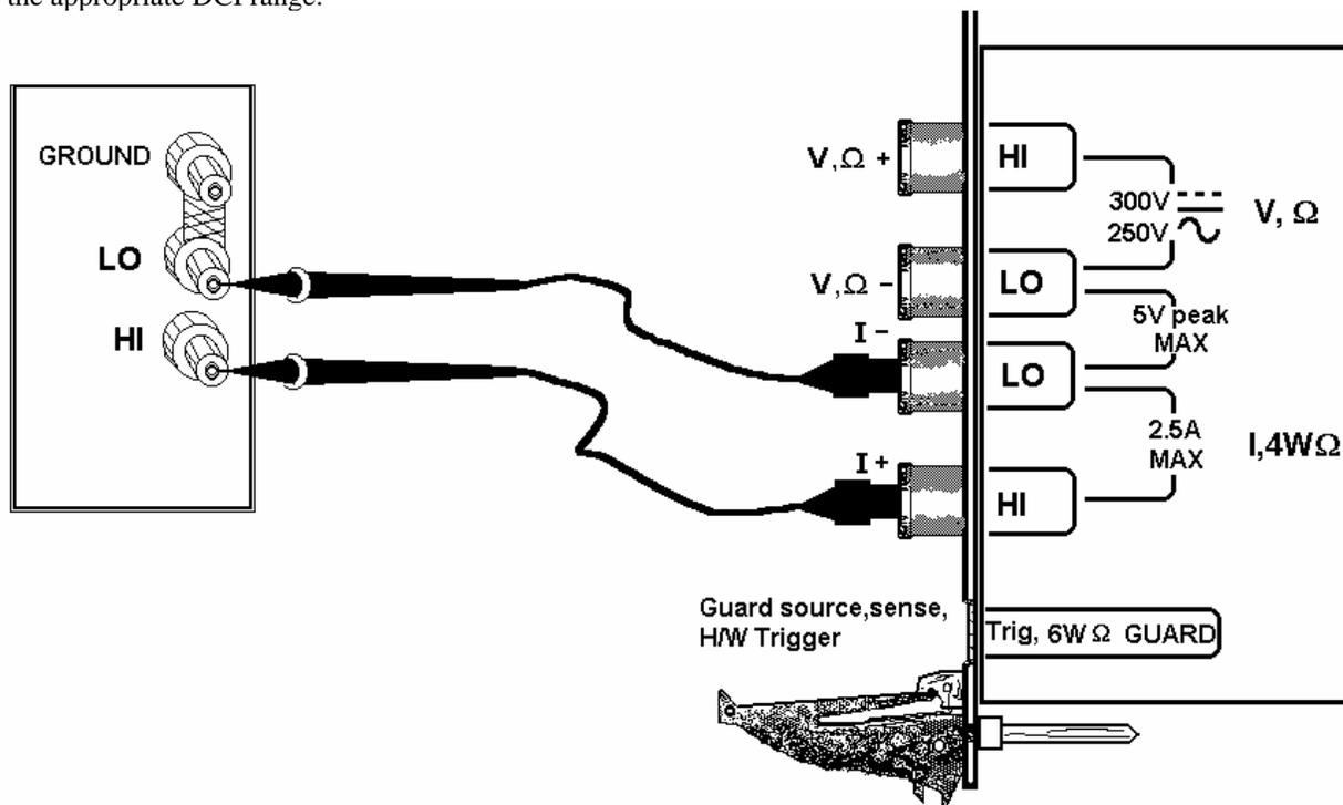
Figure 4-2. AC and DC Current measurement connection.
