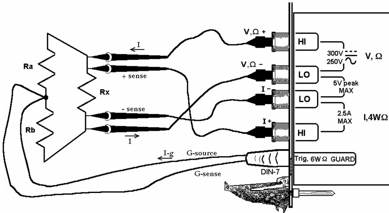
Figure 4-4. 6-wire guarded in-circuit ohms measurement configuration.
