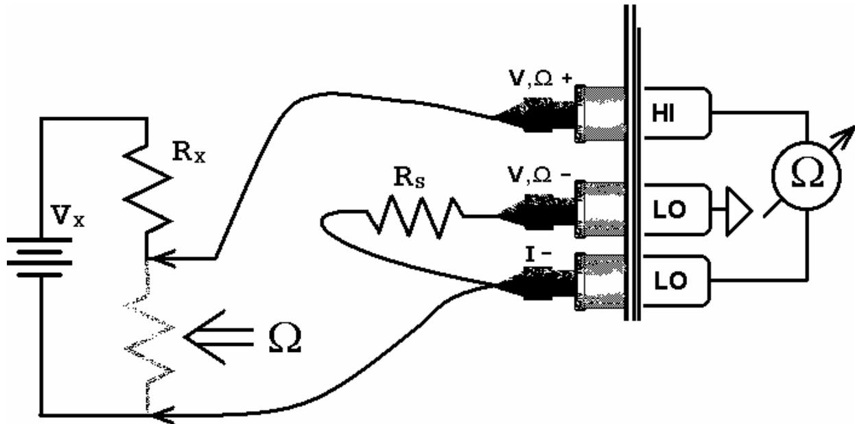
Figure 4-17. Synthesizing resistance into a voltage divider circuit.
