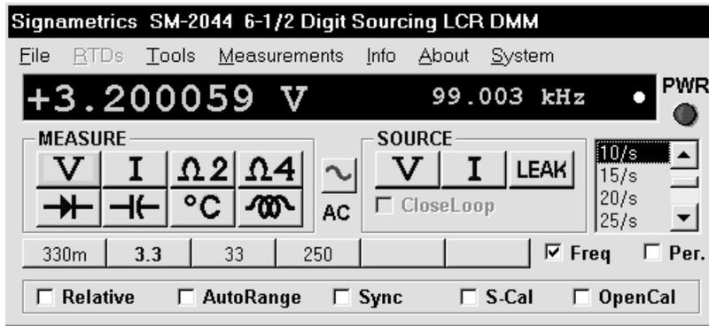
Figure 3-2. The Control Panel for the SMX2044. The three main groups include Measure, Source and Range buttons. The 8 Range buttons are context sensitive such that only “330m, 3.3, 33 and 250” appear when in AC Voltage Functions, “3.3m 33m 330m 2.5” appear when in Current Functions, etc.
