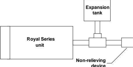
The diagram illustrates the correct installation of an expansion tank. On the left is a rectangular box labeled "Royal Series unit". A horizontal line connects it to a smaller box labeled "Non-relieving device". Above this line, between the unit and the non-relieving device, is a vertical line that connects to a box labeled "Expansion tank".
