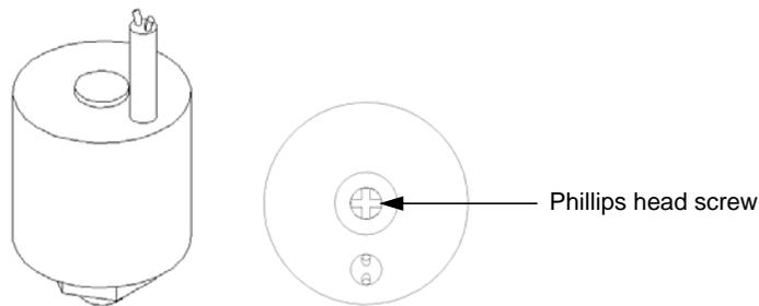
Under the plug is a Phillips-head adjusting screw:
