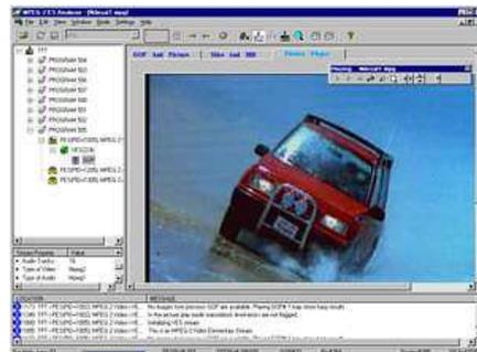
Macroblocks can be selected and detailed coding investigated. The picture analysis can be performed with special displays of quantizer scale distribution, slice size distribution, macroblock-size spectrum and motion vector plots.
