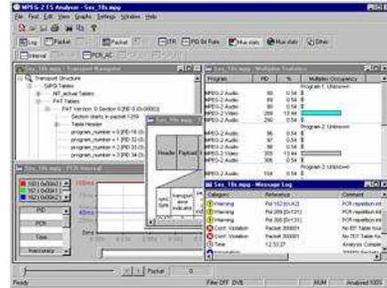
**Packet Display and Analysis** - Transport stream packet header interpretation and adaptation field information for individual packets. Hexadecimal representation of transport stream packet header and payload information. Location of a transport stream packet to match a particular condition in the packet header.
