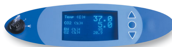
Digital O 2 display to 0.1% on 3-gas Ultima II incubators.
