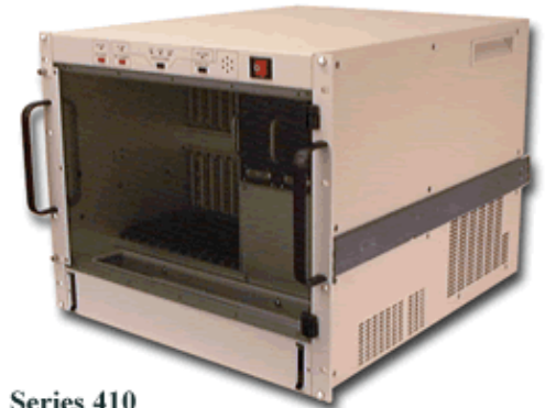
Series 410 Chassis with monitor panel 12 slot VME backplane Smoked polycarbonate door and chassis slides. Plug-in power supplies, N+1 & hot swap
