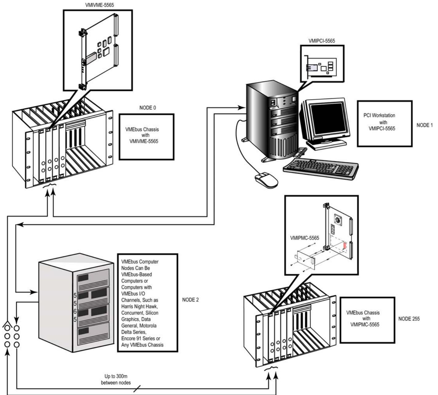
Figure 2. Network Example Using Reflective Memory System
