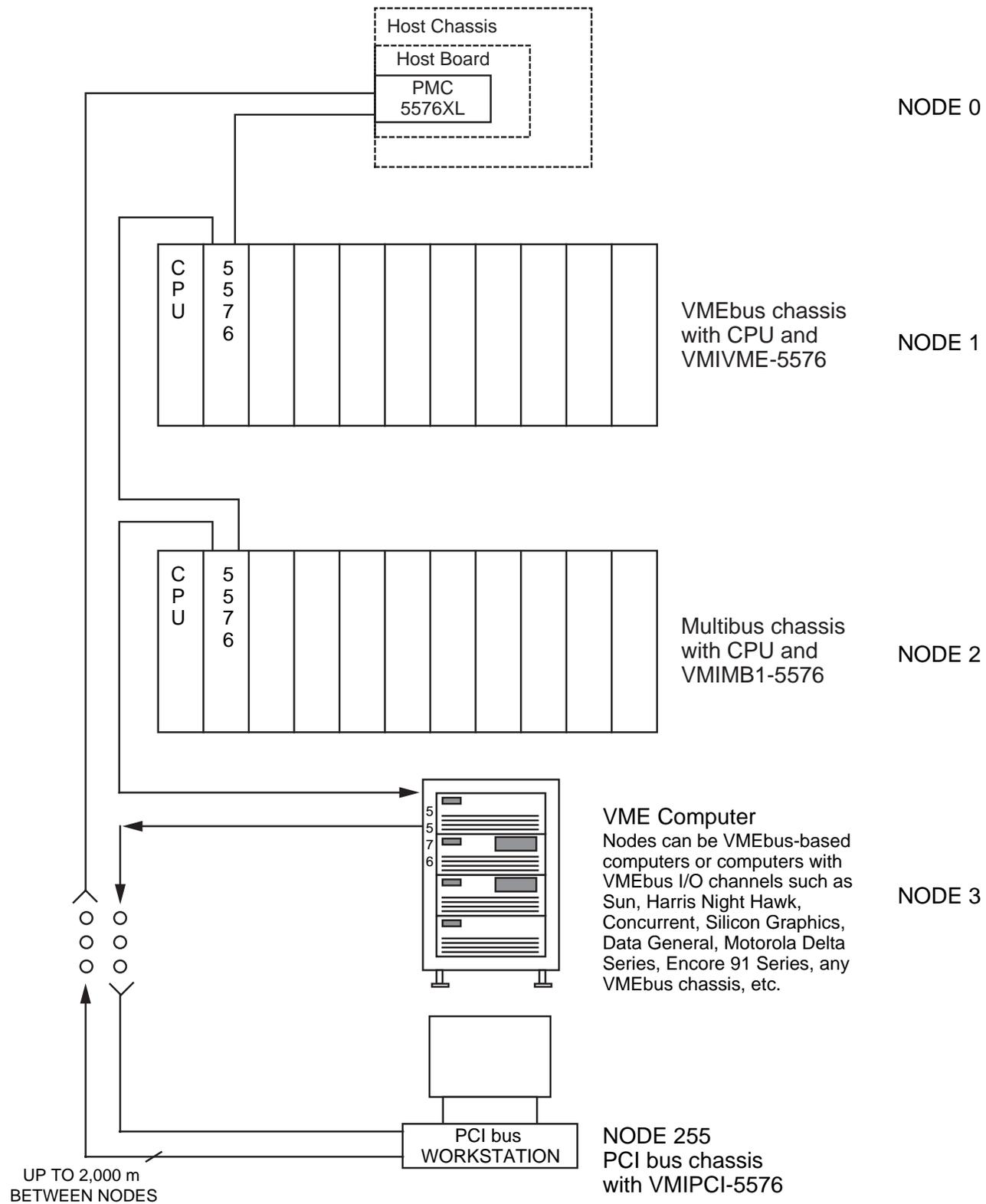
**Figure 2. Network Example Using Reflective Memory System**
