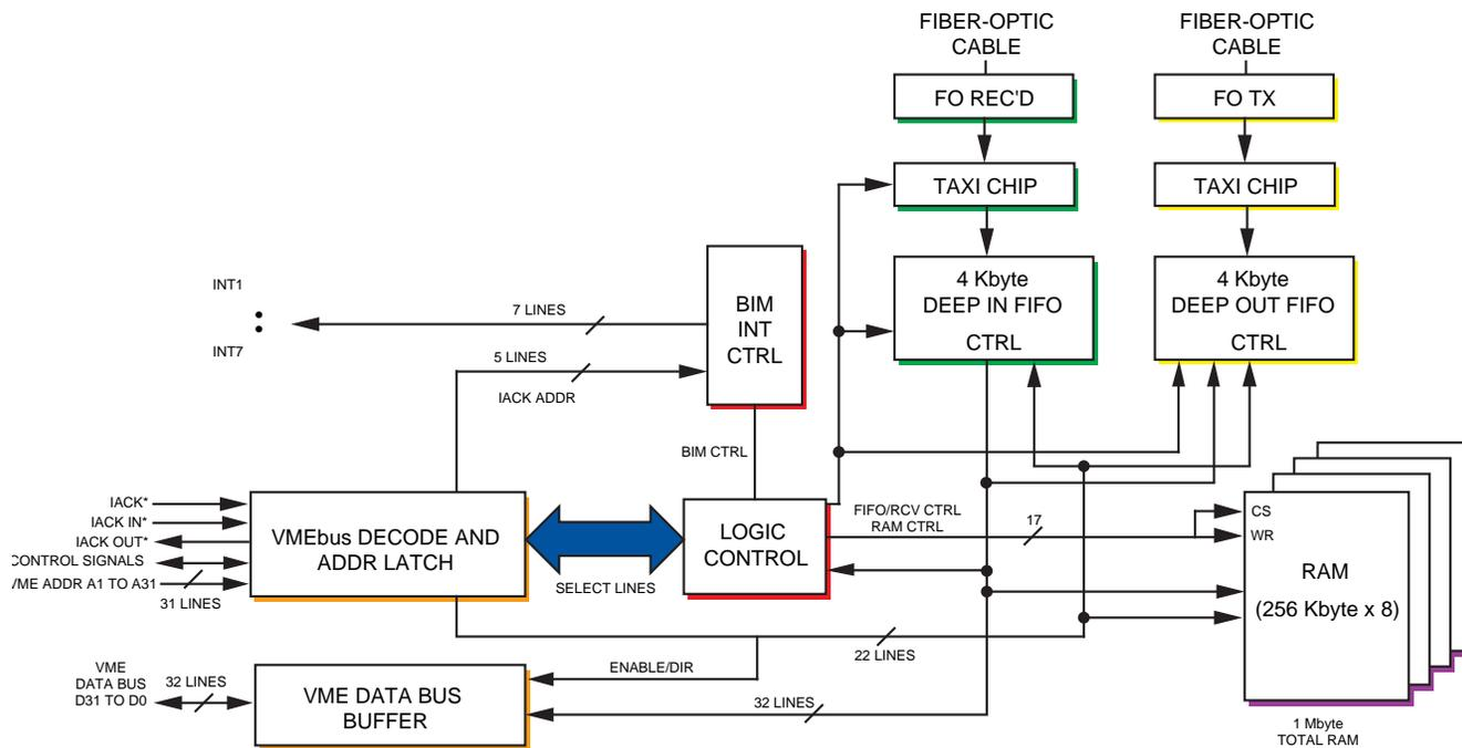
Figure 1. VMIVME-5576 Functional Block Diagram
