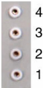
**Test Jack 4:** Internally connected to +12 volts DC (via Pin 4 of J4 on the mother board). Total current load should not exceed 75 mA.
