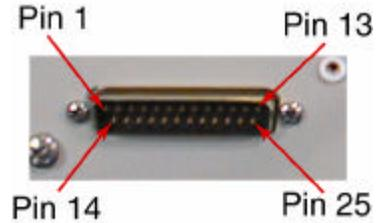
**Pin 5:** Internally connected to +12 volts DC. Total current load should not exceed 75 mA.
