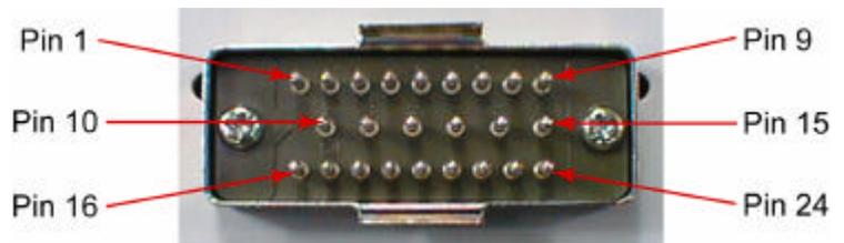
This connector is the more versatile of the two bonder interface connectors on the rear panel. It allows the bonder to directly control the power and time, without reference to channels. The bonder can also control the rate of onset of the ultrasonic power by varying the power setting during a bond.
