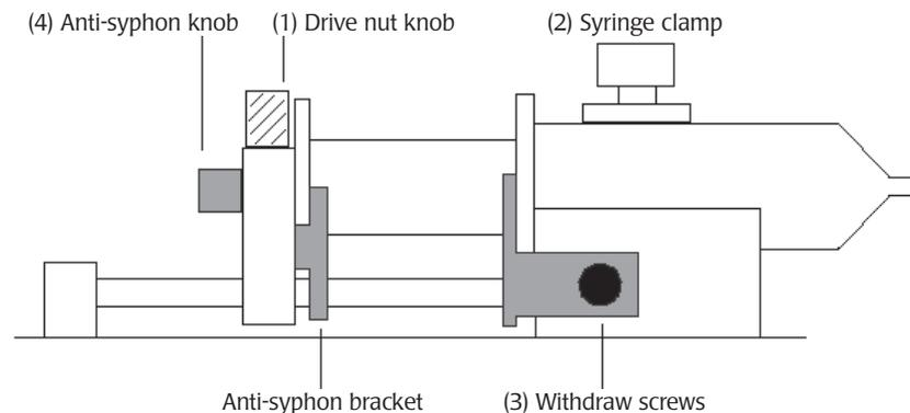
To simplify syringe loading, the pusher block can be disengaged from the leadscrew by turning the knob(1) and manually moved along the guide rods. Alternately, the Fast forward, Fast reverse feature can be used (press Run and respective Arrow key simultaneously).
